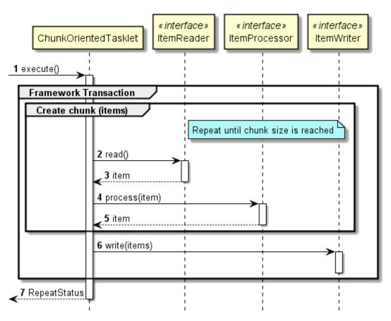
Chunk processing by using ChunkOrientedTasklet
