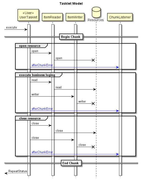
Schematic diagram of exception handling in the tasklet model
