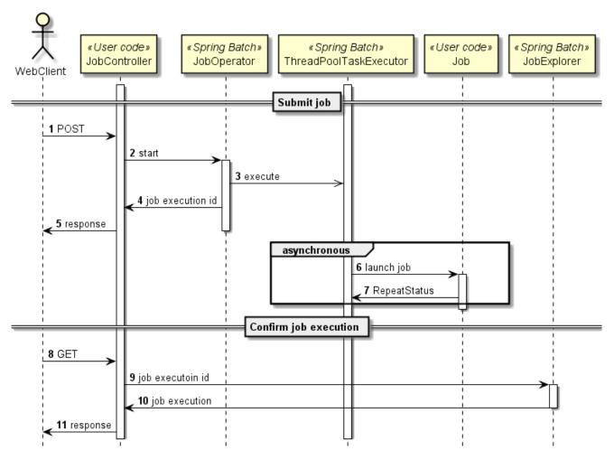
Sequence diagram of asynchronous execution (Web container)
