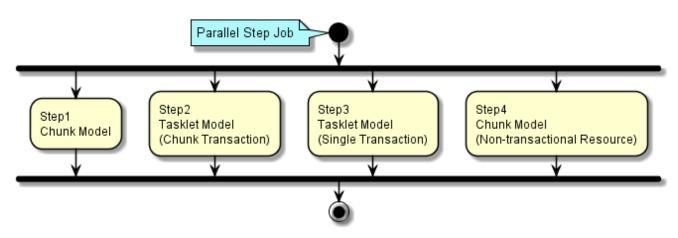
Schematic diagram for Parallel Step
