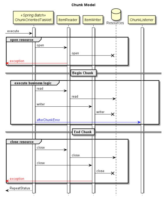
Schematic diagram of exception handling in chunk model
