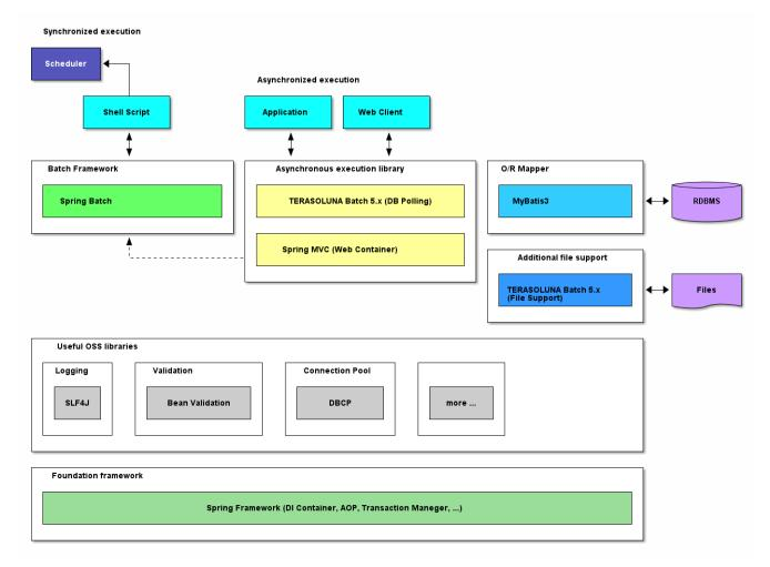
Schematic diagram of Software Framework structural elements
