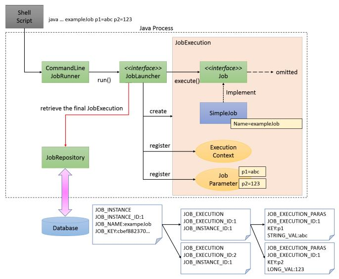
Process flow from starting a Java process till starting a batch process
